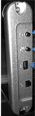
Brightness: Default set to 100%, push to adjust. To extend the amount of time between battery charges push 3 times to adjust to 25%.
